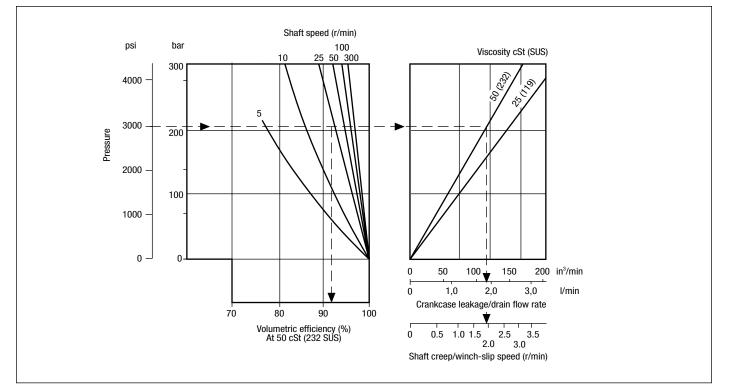
This nomograph enables the average volumetric efficiency, crankcase (drain) leakage and "winch slip"/shaft creep speed to be estimated.
