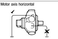
The crankcase drain must be taken from a position above the horizontal centre line of the motor.
