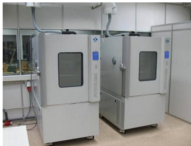
Two FitoClima chambers with liquid nitrogen injection, allowing up to 10°C / minute cooling speeds
