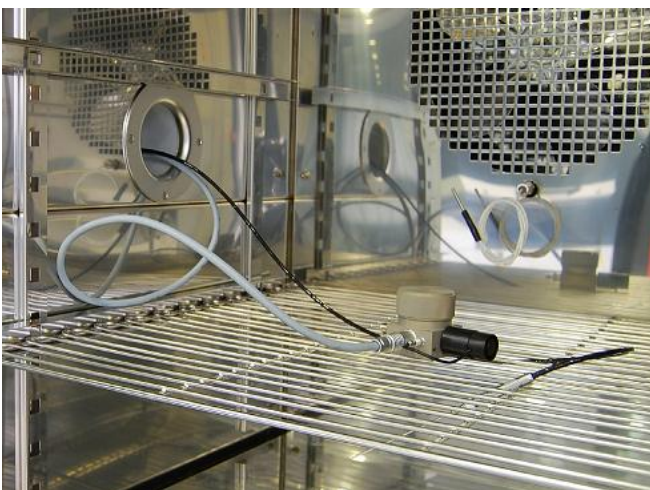
FitoClima 300 with a chilled mirror dew point hygrometer for calibration inside
