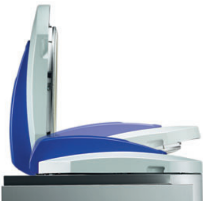
Lid closed, circumferential locking ring in lock position. The internal steam pressure presses the lip seal between lid and chamber.
