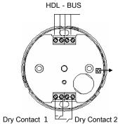
Module Indicator, flickering when the module is working fine. Keep pressing for 3 seconds, user can read and modify the address of the module in the HDL-Bus software.
