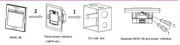
**Installation:** Hold the edge of MHIC.48 (shown as above), insert the power interface module vertically. Do not push this module too hard.
