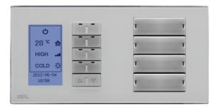
HDL-MPL8.48 8-button multifunction LCD switch is a new generation of wall-mounted switch with new design. It has 8 control buttons and the left & right side of the button can be programmed separately. There are 2 buttons are used for the page switching. Each button can display an icon in the LCD screen and the icon can be customized for final user.
