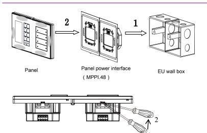
Installation: Hold the edge of panel, (see pictures on the left) ,insert the power interface module vertically. Do not push the panel too hard.
