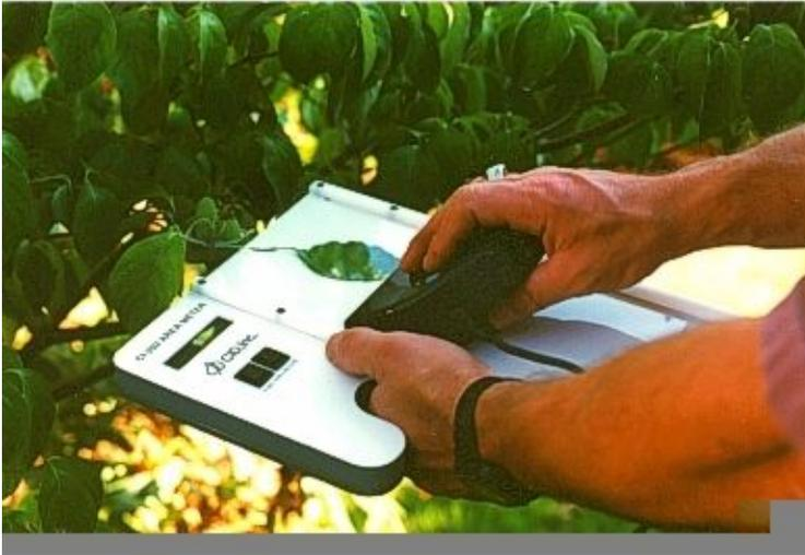
The CI-202 Portable Area Meter is one of the most affordable leaf area meter in the world. It consists of a high-speed scanner and a scan board with a built-in data logger, display, function keys and rechargeable batteries. The scan board also has guide rails and a transparent film attached for smooth scanner movement.
