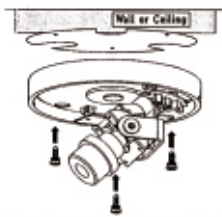
Fix the surface mount bracket by screws on the pad
