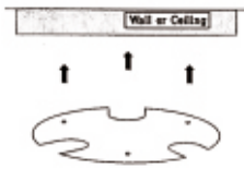
Stick a pad for free-screwing
