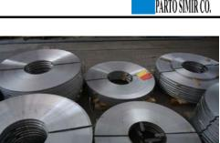
We offer a full range of Stainless Steel Banding 1/2" (13mm) 3/4" (19mm) , 5/8" (16mm) and 1" (25mm) from stock in both Bright finish (BA) and a matt finish (2B) other widths can be produced to order within short lead times typically 40mm , 50mm 75mm and 100mm. All materials are produced in catch weight coils (approx 15kg - 25 kg coil ), palletised . We are able to arrange express delivery according to client order .
