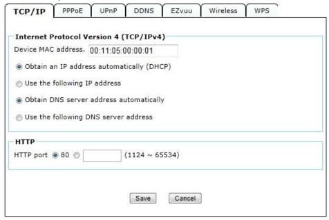
**Use the following IP address:** Select this option when the fixed IP address is set.
