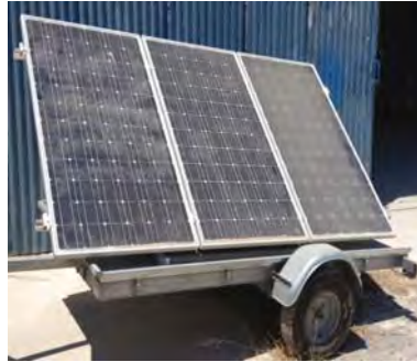
Portable PV panel after 6 months of exposure to natural environment. The difference of right module (untreated) with the other two (SurfaShield G treated) is obvious.
