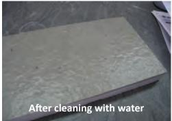
SurfaPaint Stone Varnish WB treated stone was stained with red wine, olive oil and coffee. 24 hours after the application, the stains disappeared just by using with tap water and kitchen paper.
