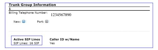
Since there are 16 active SIP lines, the number of V-SIPGW ports to be set as an"additional channel for channel 1"will be 15 ports
