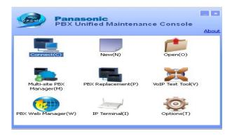
Click Connect and choose the method of connection using either LAN, RS-232, Modem, or USB to Connect to your PBX for interactive configuration
