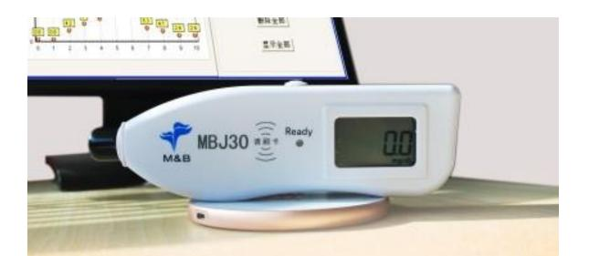
MBJ30 is a handheld instrument used in the dynamic clinical examination of neonate jaundice. It tests transcutaneous bilirubin that is correlative with serum bilirubin concentration non-invasively and instantly through placing it on neonatal skin, which will prevent the neonates from any discomfort brought by blood drawing. Meanwhile it reduces test costs and increases the working efficiency of doctors and nurses.
