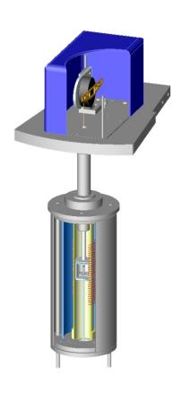
Simultaneous measurement of DSC and TGA
