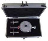
The instrument provides an accurate guide to determining the right period for fruit harvesting and monitors maturation progress during cold storage (pulp softening).
