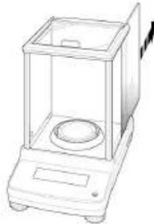
Fig. 2: Remove the glass doors
