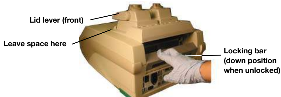
Figure 4. Inserting the reaction module into the bay.
