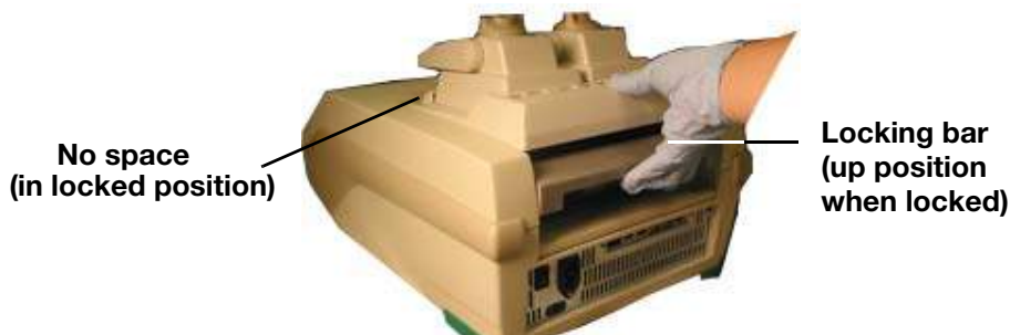
Figure 5. Locking the reaction module in place.
