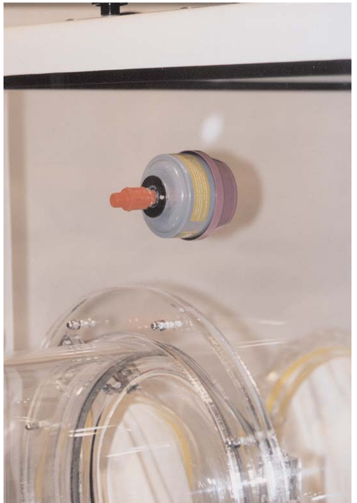
Close up view of new filter mounted inside #830-ABC (black cylinder not shown)
