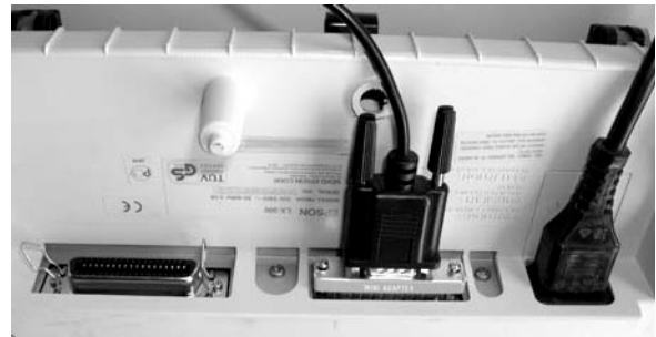
Printer LX 300 from the bottom side with IR module and adapter
