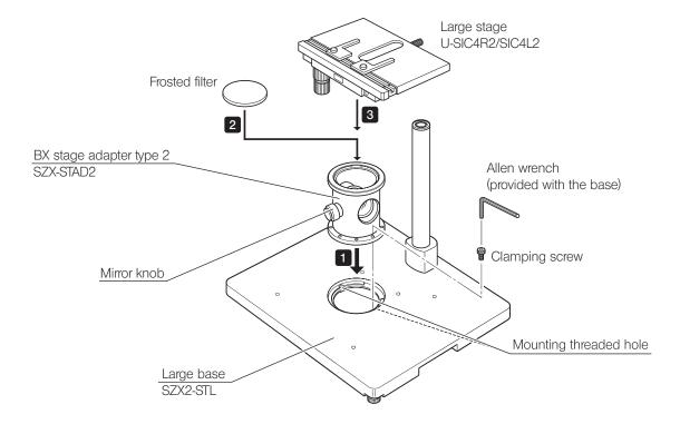
( NOTE ) For simplified transmitted light observation, place the mirror knob on the front and use a frosted filter.
