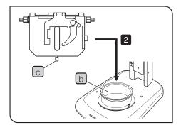
2 Place the stage clamping knob c of BH2-SH (horizontal knob stage) on the front of the base, rotate the clamping knob c in clockwise direction to secure it, and attach BH2-SH.
