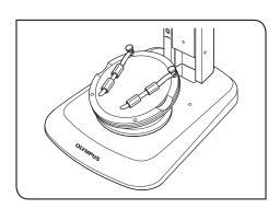
To fix a container such as a petri dish, insert the provided tube into the specimen holder to fix the container by pinching.
