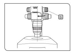
2 Return the microscope body to the illumination light path by loosening the focusing module clamping knob b, rotating the microscope body gently in the direction of the arrow, aligning visually the objective with the illumination light path and tightening the clamping knob b again. Now the setting of the photo light path is complete.
