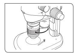
Hold the objective and gently rotate it until a click position on the front, where the objective to be used is engaged in the light path.
