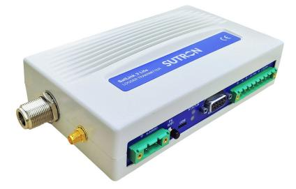
Cost-effective solution to log and transmit data over geostationary environmental satellites.
