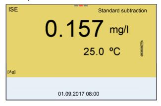
16. If necessary, start measuring further samples with **<ENTER>**. Repeat steps 6 - 15 for all samples.
