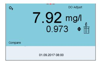
6. Using <▲> <▼>, set the correction factor to adjust the displayed concentration value to the nominal value (value of the comparison measurement). Subsequently, accept the correction factor with <ENTER>. The meter switches to the measured value display. The status display [Factor] is active.
