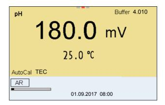
Wait for the measurement with stability control to be completed or terminate the stability control and take over the calibration value with ENTER>.
