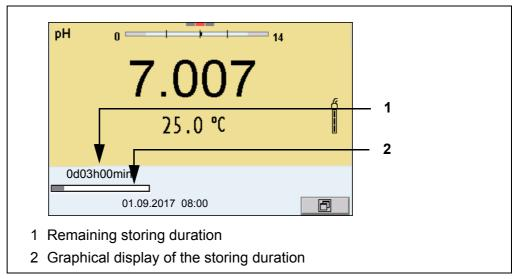
The active automatic data storing function can be recognized by the progress bar in the status line. The progress bar indicates the remaining storage duration.
