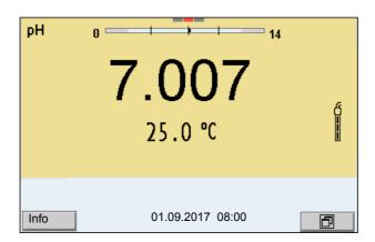
2. Open the *Storage & config* menu with **<ENTER\_>**. The instrument is in the setting mode.
