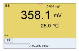
12. Wait for the end of the AutoRead measurement or accept the calibration value with **<ENTER>**.
