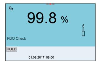
4. Start the measurement with **<ENTER>**. The measured value is checked for stability (stability control).
