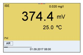
17. Wait for the end of the AutoRead measurement or accept the calibration value with **<ENTER>**.
