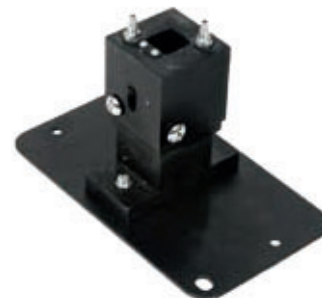
Cat. No. 18900335 10mm water-jacketed (for SCI-V1100 & SCI-UV1100)
