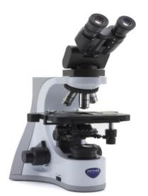
Binocular ERGO brightfield microscope, 1000x, IOS W-PLAN objectives
