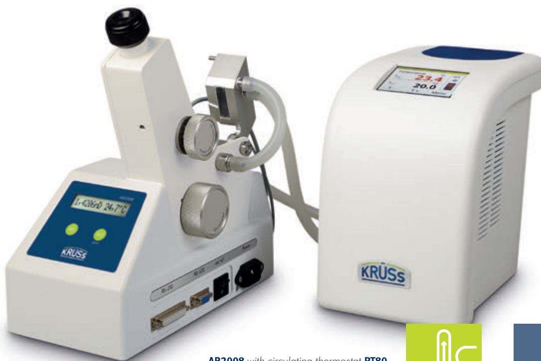
AR2008 with circulating thermostat PT80
