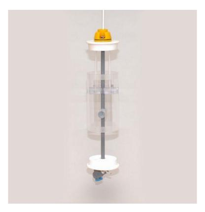
The Kemmerer water sampler (vertical sample bottle) is used for general water sampling in lakes, channels, wells and the sea. This sampler is made entirely out of plastic parts so that there is no risk of the sample coming into contact with metal. It holds 1.2 liters.
