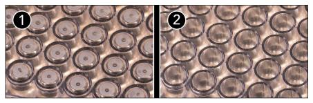
Condensation Control<sup>™</sup> sets a temperature gradient from top to bottom to prevent condensation on the sealed plates that can cause light scatter and reading artifacts. (1) Condensation on plate seals can cause inaccurate and inconsistent measurements. (2) Condensation Control in the LogPhase 600 prevents condensation, enabling consistent data collection throughout the kinetic run.
