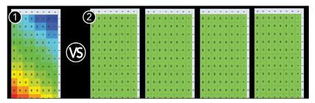
Consistent temperature control is essential to successful microbial growth assays. Incubation in the LogPhase 600 is controlled by several sensors to ensure even heating throughout, without edge effect or evaporation. Incubation can be inconsistent in some microplate readers (1). LogPhase 600 ensures consistent inter- and intra-plate heating (2).
