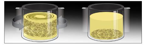
The shaking mechanism in LogPhase 600 is specifically designed for microbial growth assays; its robust and superior shaking ensures that your cells will not settle, even during long term kinetic assays.
