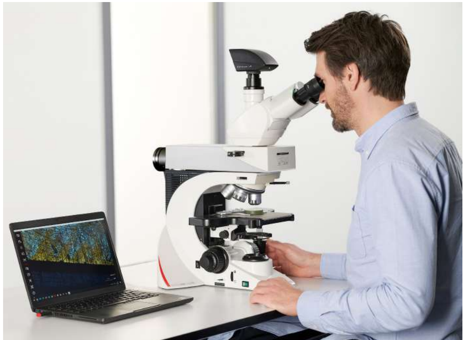
DM2700 M compound microscope with Flexacam c5 camera using the Desktop app of the Enersight software platform.
