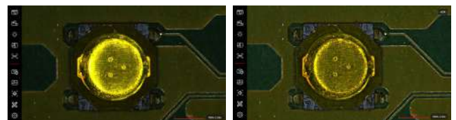
Left: Image of an electronic component without HDR Right: Image of an electronic component with HDR
