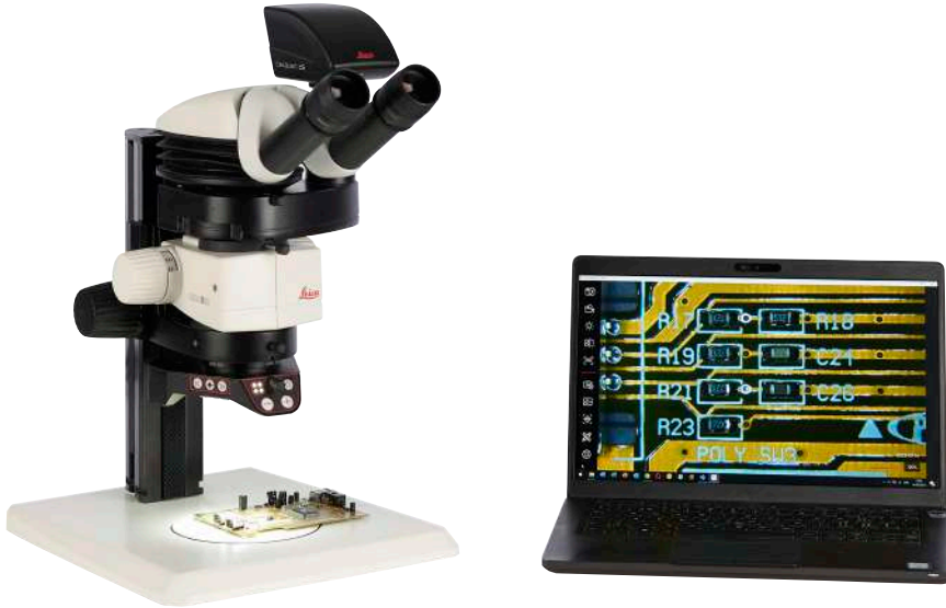
Flexacam c5 camera with M60 stereo microscope using the Desktop app of the Enersight software platform.
