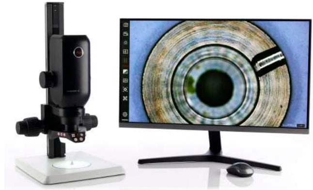
Emspira 3 digital microscope operated with the on-screen display (OSD) of the Enersight software platform.
