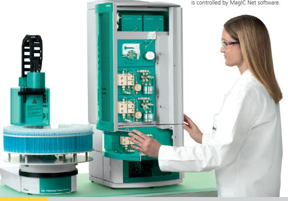
Samples can rarely be injected directly without any preparation. With the Metrohm Inline Sample Preparation techniques «MISP», sample preparation can be completely integrated into your 940 Professional IC Vario system. Some of these extended systems use the 942 Extension Module Vario LQH or the 942 Extension Module Vario Prep 2 for filtration, dilution, dialysis or preconcentration in the low-pressure range.
