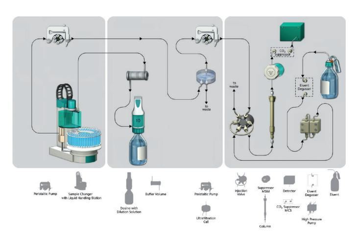
ProfIC Vario 6 Anion: IC system with sequential suppression for anion analysis after Inline Dilution and Inline Ultrafiltration. This system is fully automated and manages the most frequently used sample preparation techniques in routine analysis. It can be calibrated with a single standard.
