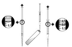
Note: to measure exactly 0.2 mL of sample with the syringe. push the plunger completely into the syringe and insert the tip into sample. Pull the plunger out until the lower edge of the seal is on the 0.0 mL mark of the syringe. Insert the syringe into the vial and push the sample out until the lower edge of the seal is on the 0.2 mL mark.
