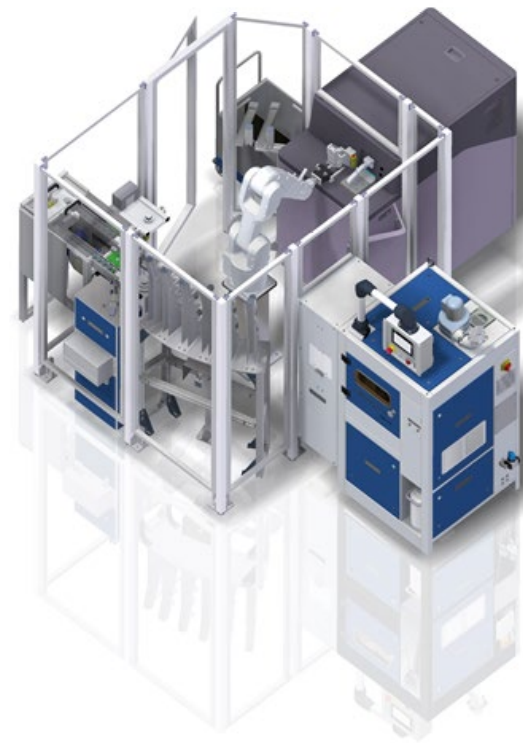
HERZOG MetalLab- The standard automation for preparation and analysis of non-ferrous samples.
