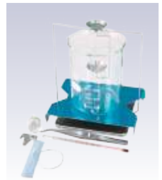
Density determination kits Make weighing the sample in air and in water quicker, easier and more precise. A&D Apollo can then perform a density calculation automatically.
