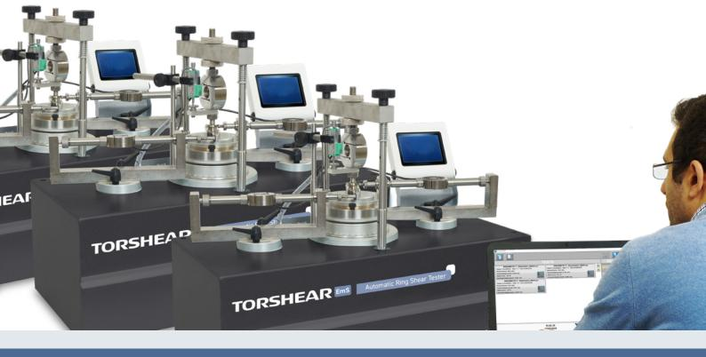
Torshear EmS is a versatile and fully automatic ring shear testing machine that benefits from the new low maintenance, efficient and environmentally-friendly Electromechanical Servoactuation (EmS) technology.
