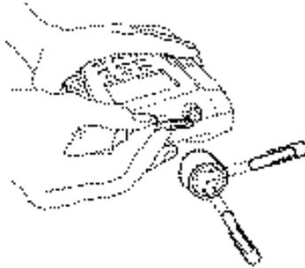
\* **Note:** Meter accuracy is  $\pm 0.1$  mV at calibration temperature, not including long term drift and a temperature error. The zero and slope temperature coefficients of the meter over the range of 15 to 40°C specify  $\pm 4$  mV at full scale (worst case). The long term drift will not exceed 0.1 mV per month.
