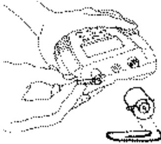
To test the meter for correct operation with a **pH Twist-lock electrode**, short the Twist-lock input connector using two paper clips as shown. Each paper clip must touch two adjacent pins inside the connector. Press **mode** and select mV mode. If the meter reads  $0 \pm 0.1$  mV\*, it is measuring correctly.
