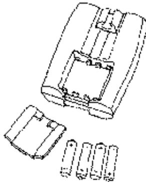
**Note:** Nickel-cadmium rechargeable batteries can be used, but their operating life is half that of alkaline cells, and they cannot be recharged in the meter.
