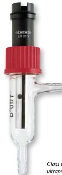
Glass flow-through vessel D01/T with ultrapure water cell LR 01 V
