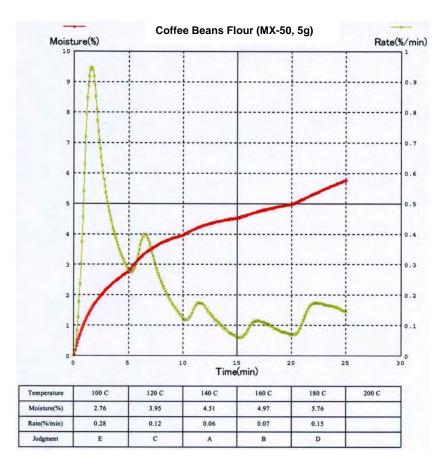
This graph shows results of measurement on coffee beans. Moisture content rate curve (red) does not stabilize to a horizontal line. The differential curve (green line) increases and decreases after the
