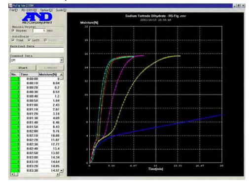
Sodium tartrate dihydrate heated from 100 °C to 200 °C at intervals of 20 °C.
