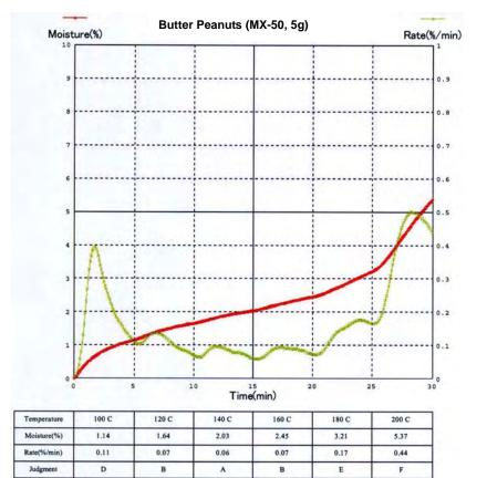
The upper and lower graphs display measurement results for soy powder and butter peanuts.
