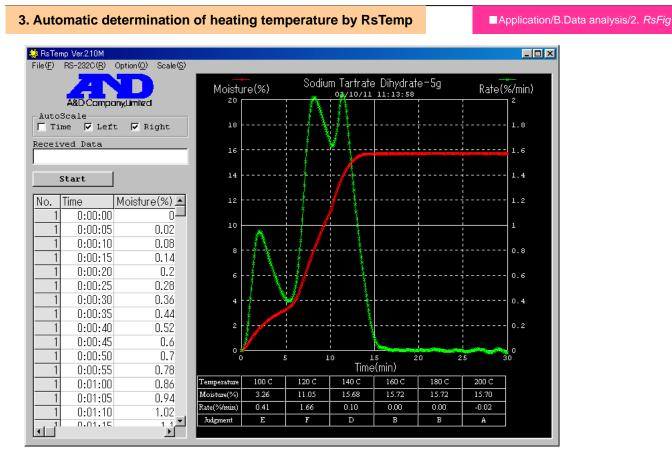
The RsTemp software determines the optimum heating temperature for measuring moisture content with the MS/MX/MF/ML.
