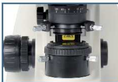
KOEHLER ILLUMINATION / SLIDING-IN ABBE BRIGHT FIELD CONDENSER
