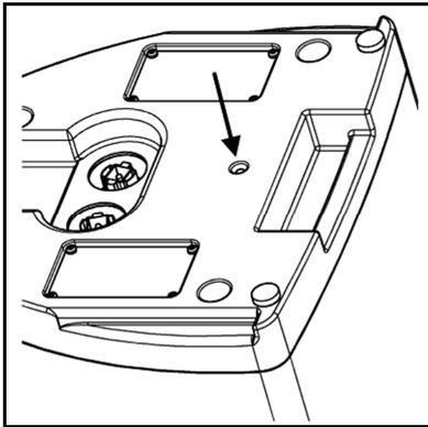
Fig. 15: Resetting the heating bath's circuit breaker
