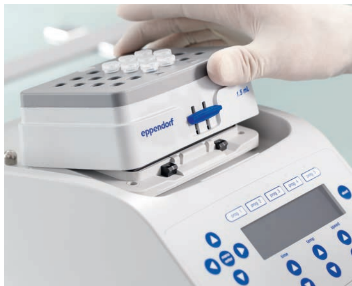
SmartBlock removal from Eppendorf ThermoMixer® C
