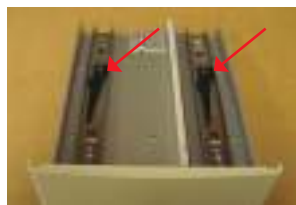
Fig. 15. Underside of the drawer. The black tabs (arrows) can be pushed to release the drawer from the tracks.
