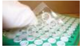
Fig. 10. Uniform and complete circles demonstrate good sealing.
