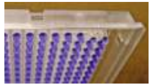
Fig. 11. Examine sample volumes after cycling. In this demo, corner wells were poorly sealed to demonstrate sample evaporation.
