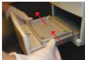
Fig. 14. Top of the drawer. Arrows indicate the direction to push the release tabs to remove the drawer.
