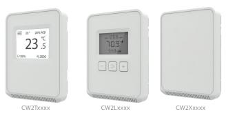
The CW2 Series of air quality sensors for living space is a flexible multi-sensor platform for use with BAS controllers designed to accept 4 to 20mA, 0 to 5Vdc or 0 to 10Vdc outputs. CW2 Series sensors are available with three user interface options: touchscreen, LCD with three buttons and blank. CO<sub>2</sub> and temperature sensors are included with all CW2 Series air quality sensors. Models with VOC sensors and relative humidity sensors are also available.
