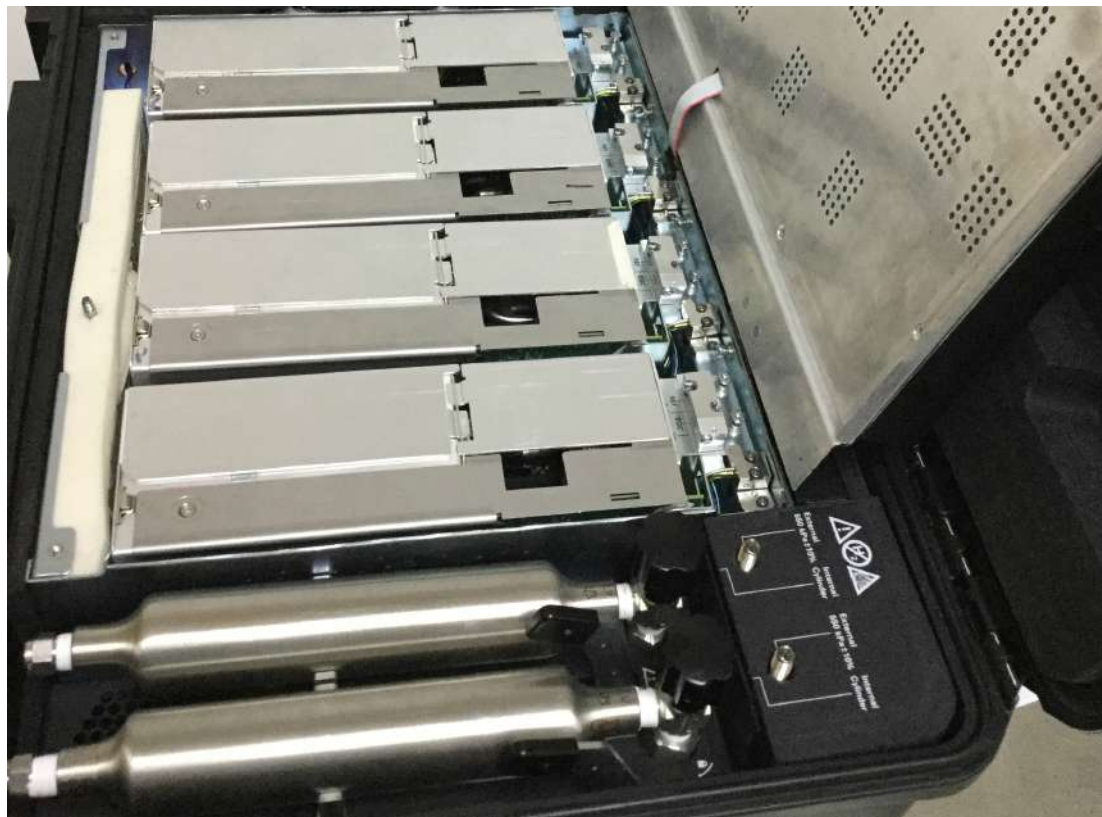
Figure 7. Inside view detail with Channels and Gas Cylinders installed
