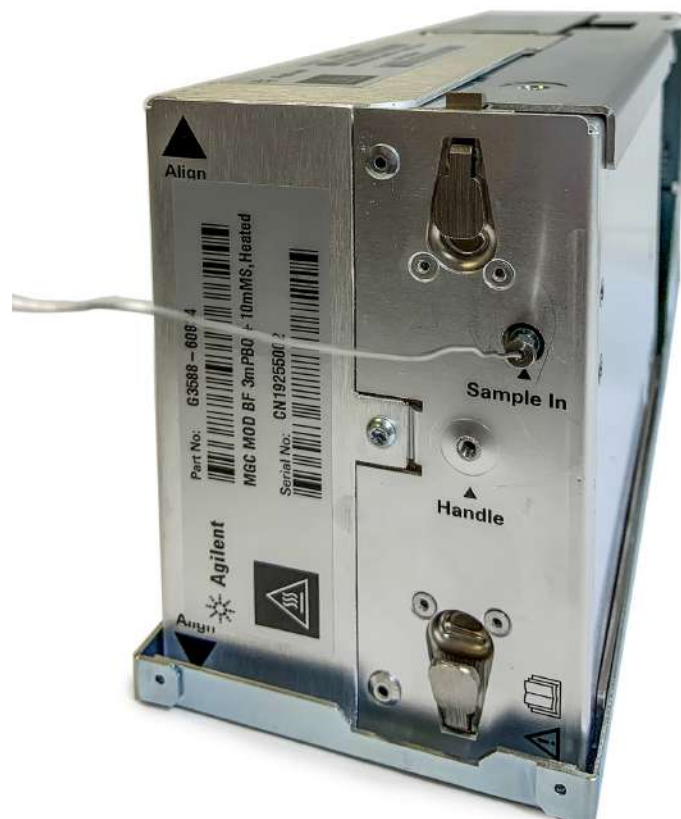
Figure 14. Sample inlet tubing connected
