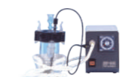
▶The mantle heater ensures the complete extraction of moisture of sugar samples.
