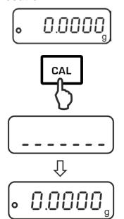
Press **CAL** button in the weighing mode.
