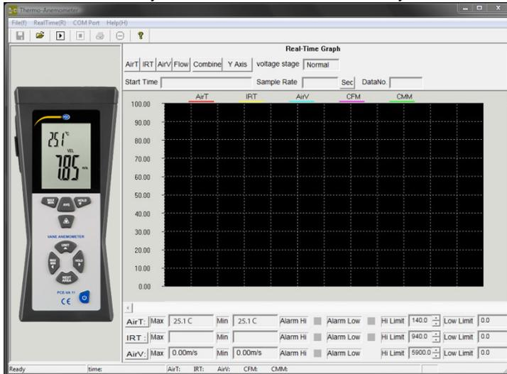
If the device is not identified by the software, make sure that the right COM port is selected. You can see the COM port of the device by checking your device manager (Windows Control Panel - > Device Manager).
