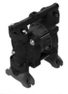
Air-operated double diaphragm pump for pumping viscous, corrosive and abrasive liquids. The plastic double diaphragm pump is suitable for pumping small quantities, in the laboratory and for occasional filling. Suction and discharge connections are 1/4" internal. Solid particles up to 3 mm Ø can be pumped. Housing, diaphragms, valve balls and seals are available in different materials. Required air pressure at start-up min. 2 bar, operating air pressure max. 8 bar.
