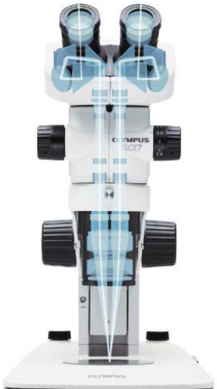
Galilean optics feature two (right/left) independent and parallel zoom optical paths. This system enables high optical performance as well as system modularity.
