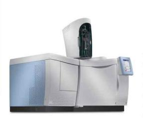
Gas Chromatography–Mass Spectrometry (GC-MS) is a method that combines the features of gas chromatography and mass spectrometry to identify different substances within a test sample.
