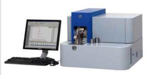
Optical Emission Spectroscopy (OES), also called Atomic Emission Spectroscopy (AES) or arc spark emission spectroscopy, is an important tool for fast and accurate elemental analysis of metals and semiconductors.
