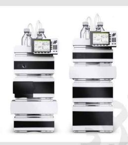
HPLC is a chromatographic technique used to separate a mixture of compounds in analytical chemistry and biochemistry with the purpose of identifying, quantifying and purifying the individual components of the mixture.
