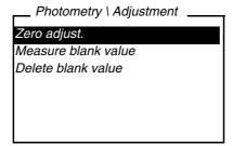
4 Using <▲> <▼> and <START/ENTER>, select and start the Zero adjust. or Measure blank value function.
