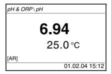
2 Press the **<M>** key (short pressure) repeatedly until the measured parameter, *pH* is selected.
