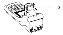
3 Open the external light cover (4) of the cell shaft.
